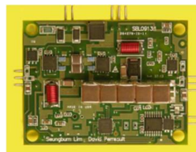
Figure 1. Microfabricated coreless inductor (left) and high frequency DC-to-DC converter (right)
