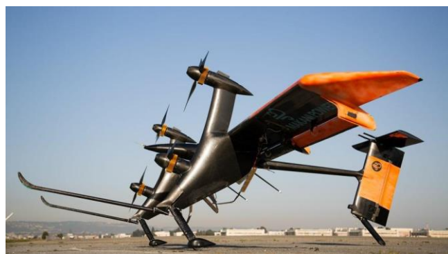
Figure 1. Makani's 20 KW (average output when flying under optimal conditions) working prototype
